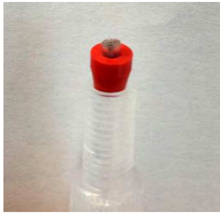
Incorrect (inner tubing protruding)
