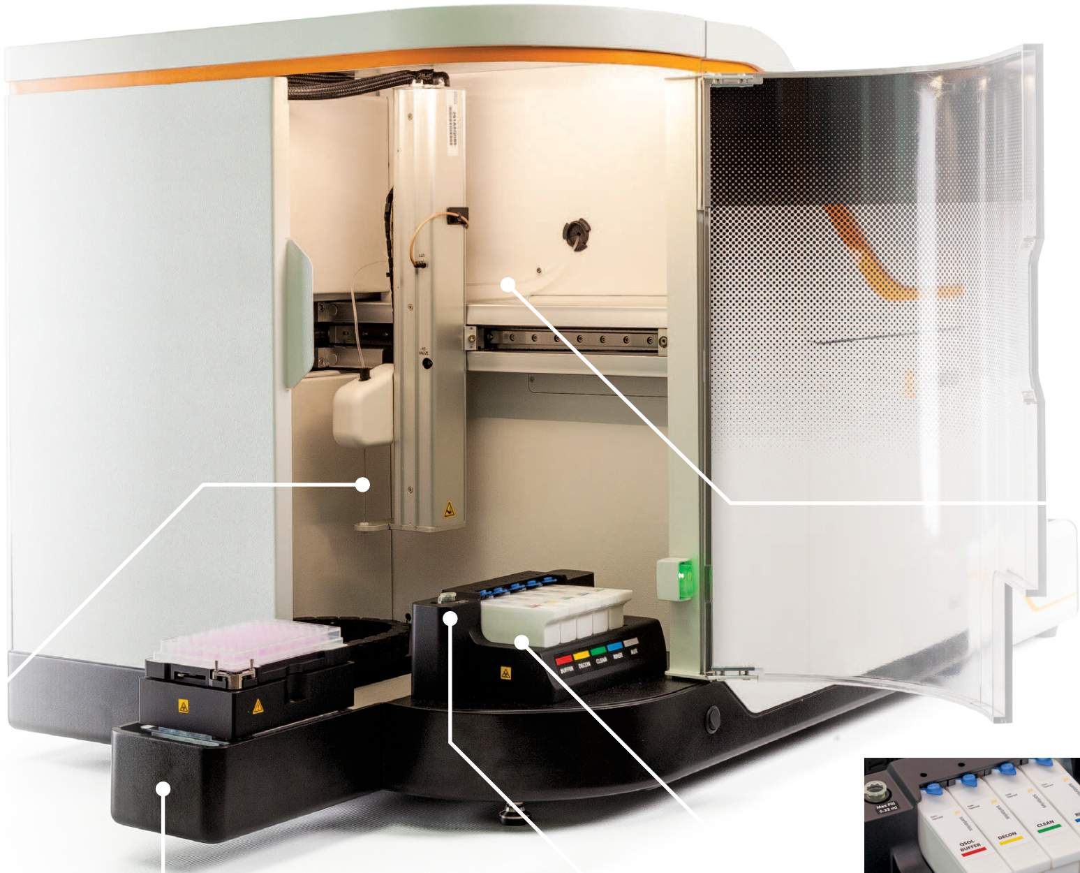
Samples are delivered to detectors in an air-gap delimited stream as part of a patented, rapid microvolume sampling process.
