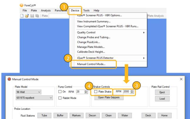
Figure 7. Steps for using the shaker on the iQue Screener PLUS and iQue3.
