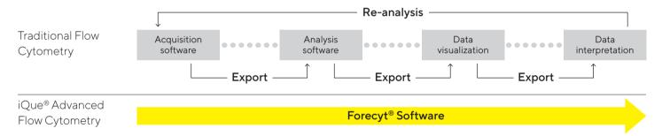
Traditional flow cytometry data analysis workflows versus one unified workflow using Forecyt® Software on the iQue® 3. Traditionally scientists have been required to export and import data between several software packages in order to go from acquisition to analysis to data visualization and even to statistical packages for interpretation of their data. Forecyt® software provides all of this functionality in a single easy-to-follow workflow to get to actionable answers in record time.
