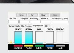
Automated data analysis and tracking of QC functionalities allows identification of potential instrument performance issues before running precious samples.
