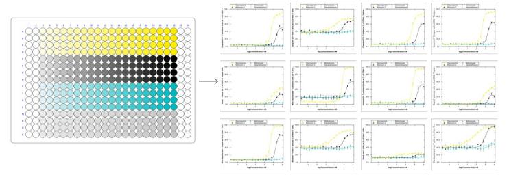
Dose-response curves for four compounds which induce apoptosis in PBMCs: PBMCs were immunophenotyped into three subpopulations and dose-response curves generated for each population for caspase positive, Annexin V positive, membrane permeability and mitochondrial depolarization using a curve fitting algorithm. Quickly generate dose response curves for all experiments across an entire plate.
